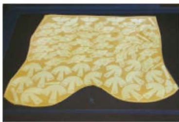
The projection of the shapes nested on the leather with EliNest
